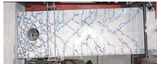
L8-8-12M-B3, F c 24, H=D/3.5, A=D/3, \tau_{mu0}/\sigma_B=0.073
