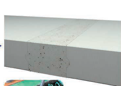
[Photo] Pouring: The concrete is poured in the spaces in between.
